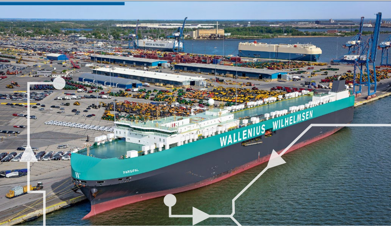
The port of Baltimore is regularly called at by the Parsifal, built in 2011. As a PCTC (pure car and truck carrier) it offers space for around 6,000 vehicles over nine decks
