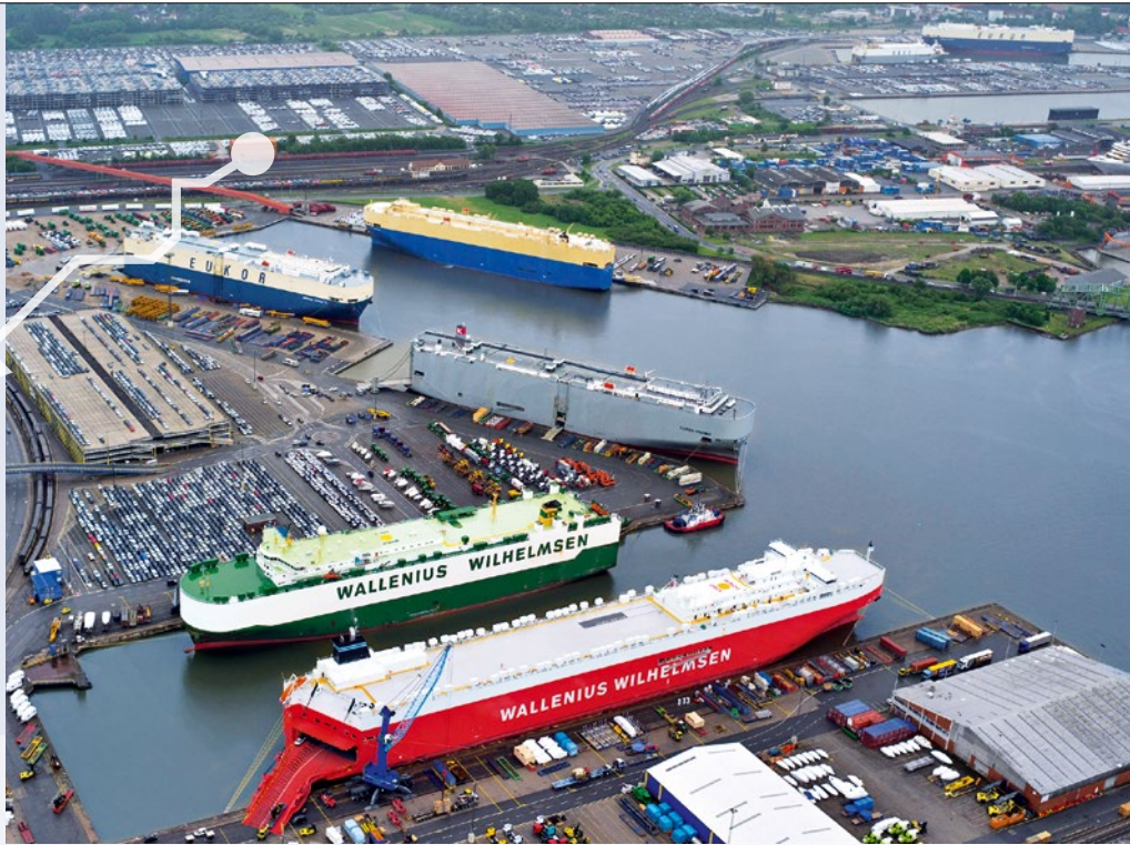
Bremerhaven boasts five RoRo berths in the Nordhafen and Kaiserhafen ports, each with a draught of eleven metres.
