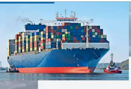
The number of tugs varies according to local conditions. For large Triple-E class container ships with 18,000 TEU, three tugs are usually required.
