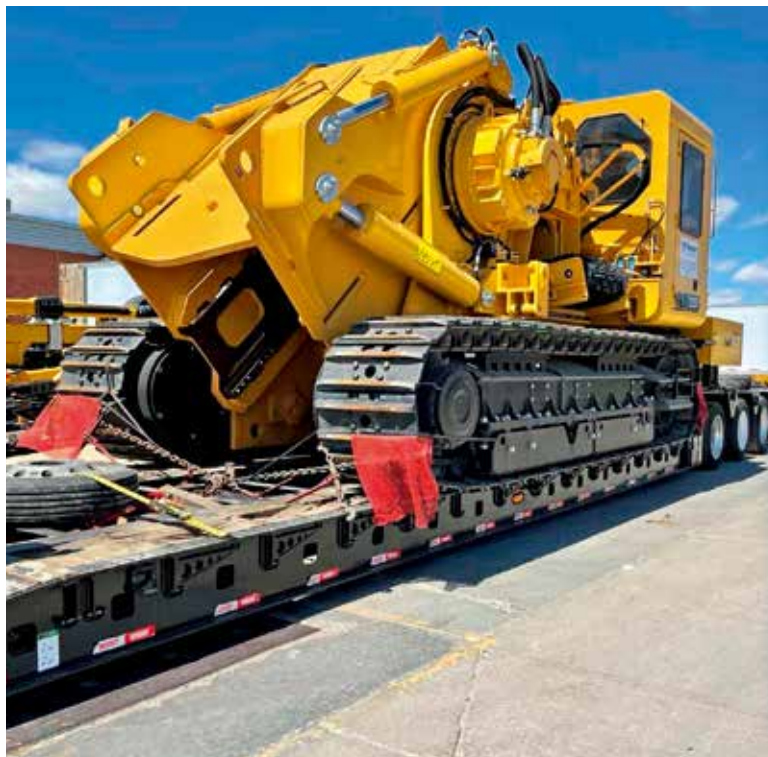
Used to dig trenches for cables, pipes or drainage, this 73-tonne trencher was recently shipped from Bremen to Libya by Carl Ungewitter.
