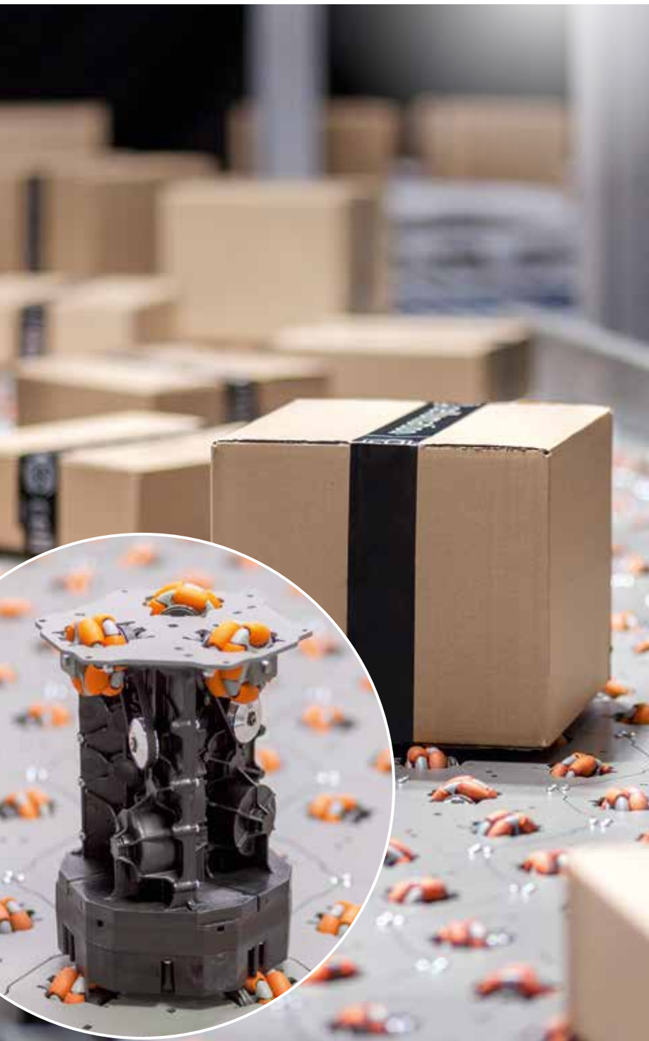
Cell-based conveyor technology enables packages to be sorted more efficiently and containers to be unloaded more quickly.
