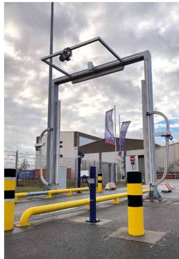
Snapshots of the status of the loading unit are taken at TriCon’s OCR gate.
