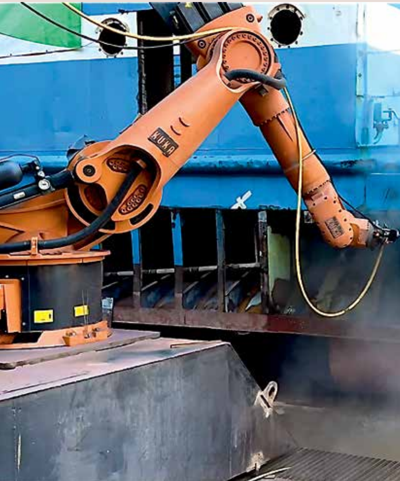
Robots in action: here a section of the ship is being cut away using high pressure and a jet of water and sand.
