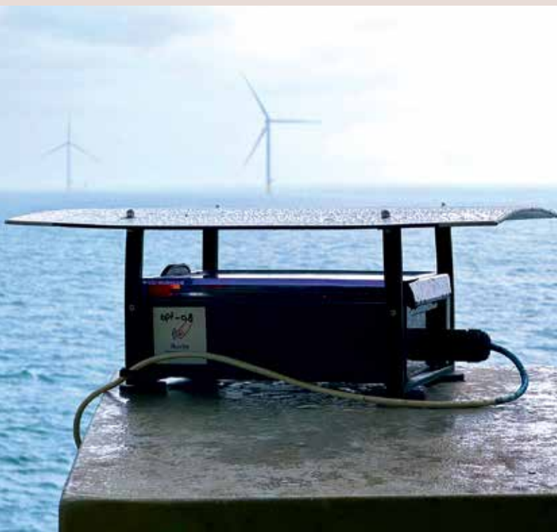
“Optical pile tracking” provides important data to make the process of installing and assembling wind power components more predictable.
