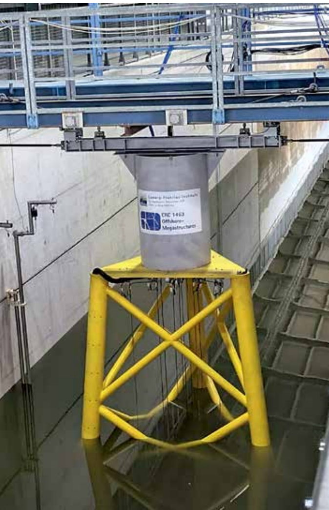
A 1:14 model of a jacket structure from the SFB. It depicts a foundation structure for an offshore wind turbine with a total height of over 300 metres.
